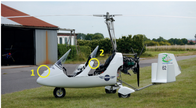
Figure 4. Gyrocopter used in the experiment. (1) GNSS - R antenna, (2) Extra GPS antenna + INS for flight control purposes.
