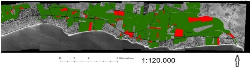
Figure 4. Location of those parcels with extreme discrepancies in area relative error. In green we show those parcels which relative area error belongs to the interval [-25\%,+25\%] and in red those with larger values. Non coloured cases denotes parcels without enough information to perform the computations. Source: Own elaboration.
