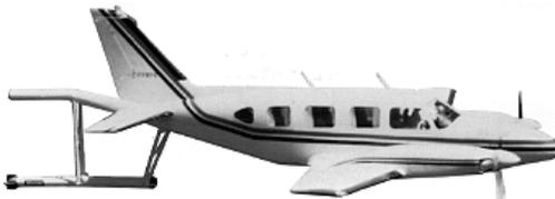
**Figure 1.** Scintrex high, sensitivity magnetic vertical gradient system.
