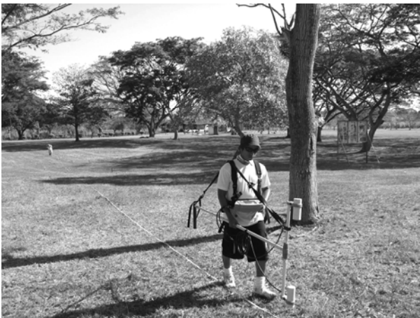
Figure 2. Disposition of the caesium magnetometer in mode gradiometer and magnetic record along a profile.
