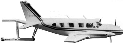
**Figure 1.** Scintrex high, sensitivity magnetic vertical gradient system.
