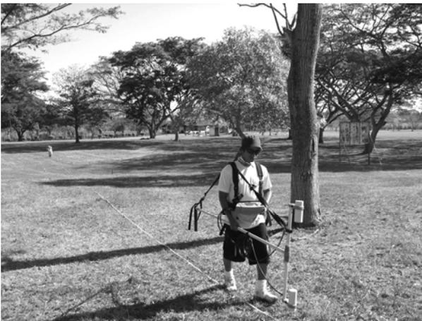
**Figure 2.** Disposition of the caesium magnetometer in mode gradiometer and magnetic record along a profile.
